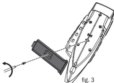
3. Use a Phillips screwdriver to open the battery compartment cover. Insert 4 x 1.5V AA batteries with the correct polarity and replace the battery compartment cover (fig. 4).
