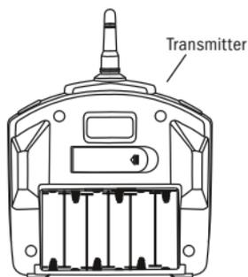
2. Insert 6 x AA batteries (not included) with the correct polarity and replace the battery lid.
