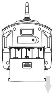
1. Slide the battery lid downwards to open the battery compartment.
