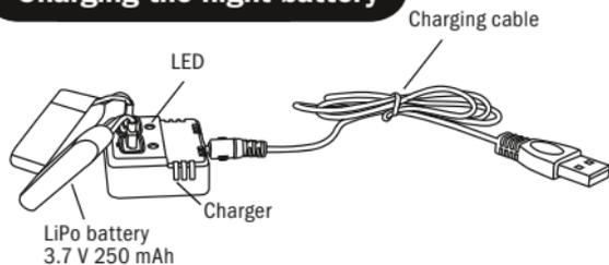
Insert the USB plug into the USB port on your computer. Insert the charging plug into the charging socket on the LiPo charger. Now insert the LiPo batteries into the charger. The red charge LED on the charger will light up to indicate the charging is in process. As soon as the red charge LED will extinguish the LiPo batteries have been completely charged.
