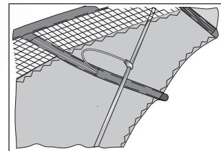
First assemble the kite as usual. Take care that all rods are inserted as far as possible into the connectors. First attach the sail battens to the wing tips on the front of the sail. To do this, insert the end of the rod with the end cap into the Dacron pocket at the wing tip. Insert the other end into the
