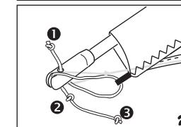
**Step 1:** Slip the loop of the hem tensioning cord (if there is one) into the slot in the split cap. Then pull the short tensioning cord through the hole in the cap so that knot 1 disappears inside the recess. Now put the other end through the knot on the leading edge, as shown in the drawing.
