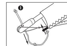
The HQ split cap makes it easier to spread the leading edge using a tensioning cord. After assembly, the knots and cord ends are tucked away inside recesses specially provided for this purpose, so that you achieve a clean finish. There's also a neat way of attaching a trick cord here.
