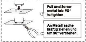
Pull and screw metal tab 90° to tighten
